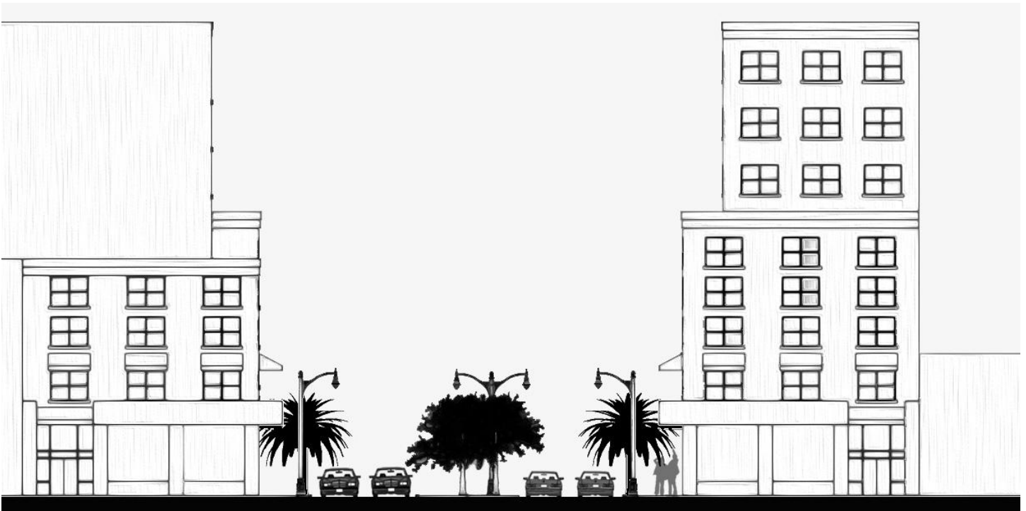
Figure 3.9: Core Street Section (SR 40, 90' ROW)
