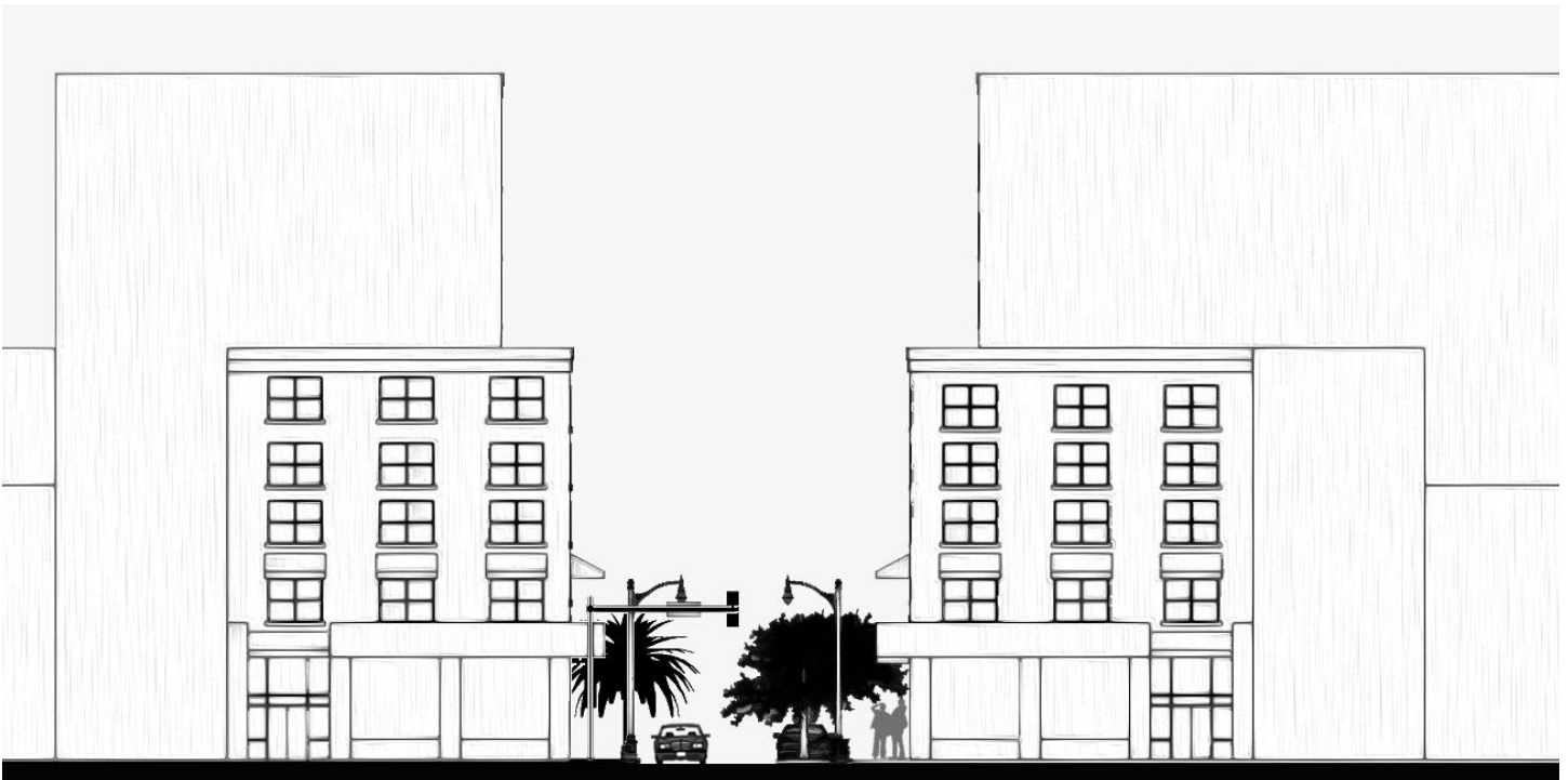
Figure 3.7: Core Street Section (50' ROW)
